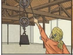
Pulleys can be used to make a small force lift a lighter load. The more wheels in a pulley, the less force is needed to lift a weight.
