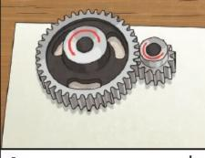
Gears or cogs can be used to change the speed, force or direction of a motion. When two gears are connected, they always turn in the opposite direction to each other.
